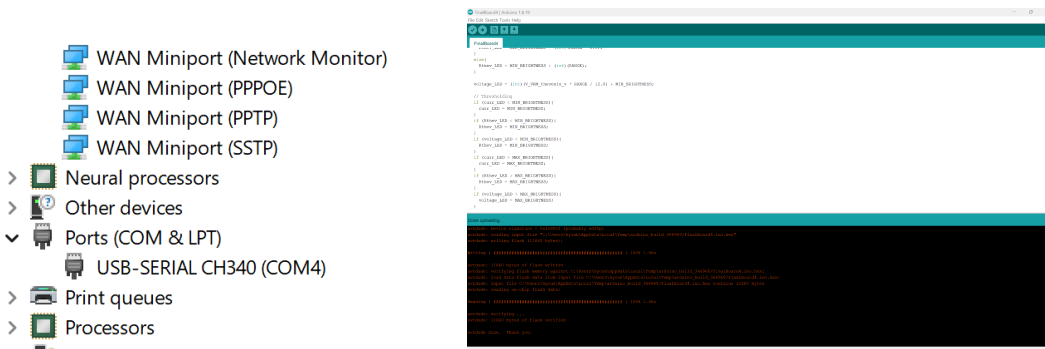
Figure 10: CH340g recognized in COM port (Left), Successful Arduino programming (Right)
