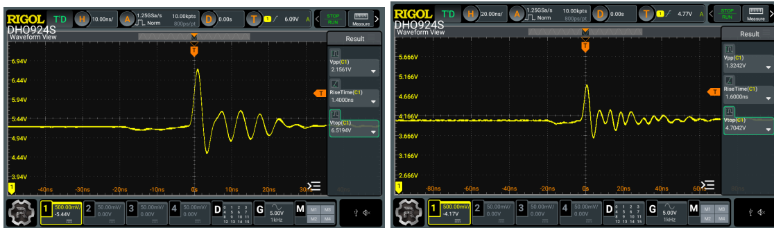
Figure 13: Quiet High Test Point (Left: no resistor, Right: 47 ohm resistor)
