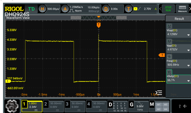
Figure 7: Output from 555 timer module without load
