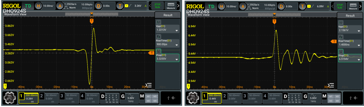
Figure 17: Quiet High Switching Noise with ground plane (Left: 3.3V, Right: 5V)
