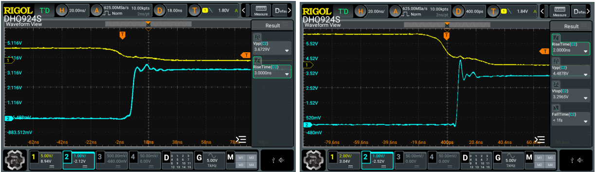
Figure 8: Rising Edge of Inverter (Left: No ground plane, Right: Ground Plane), 1V scale
