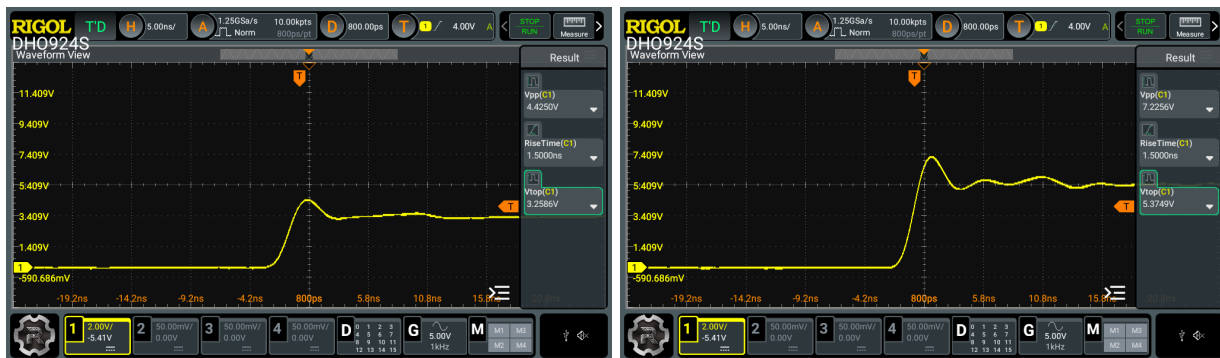
Figure 16: Rise Time of inverter with ground plane (Left: 3.3V, Right: 5V)
