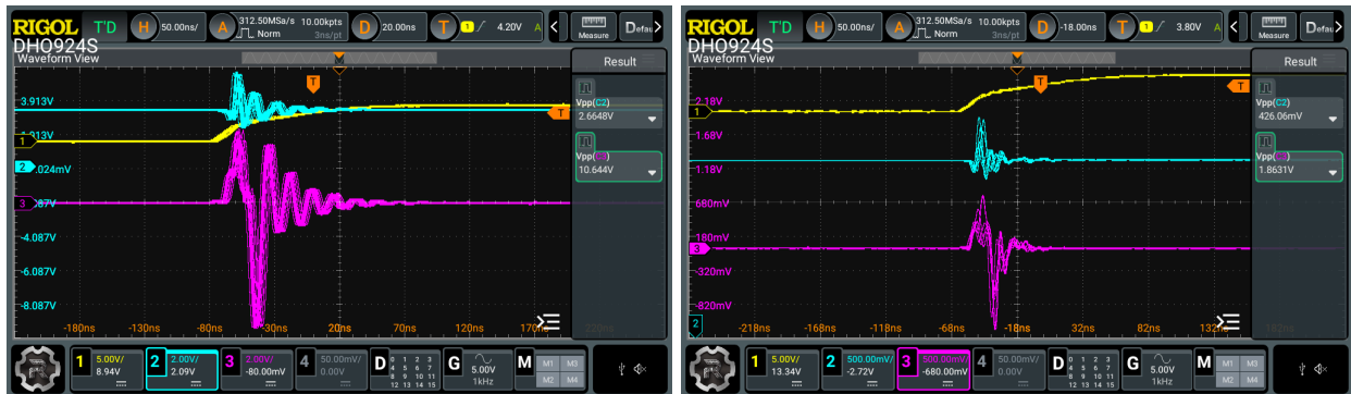
Figure 10: Quiet High/Low Noise during 555 Posedge (Left: No ground plane, 2V scale, Right: ground plane, 500mV scale)
