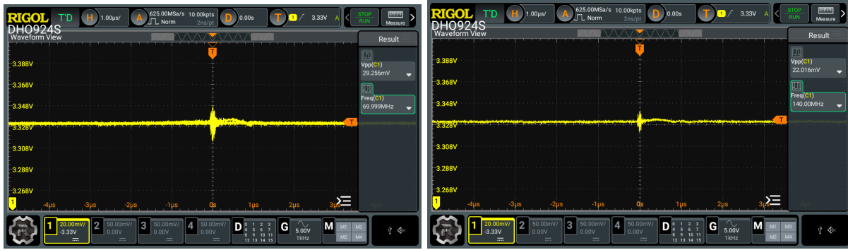
Figure 14: LDO 3.3V output oscillation (Left: with 22uF filter capacitor, Right: w/o 22uF filter capacitor)
