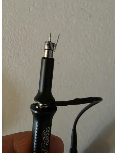
Spring Connector used in 10x Probe (left), TP1 power rail 5.5V output (right)
