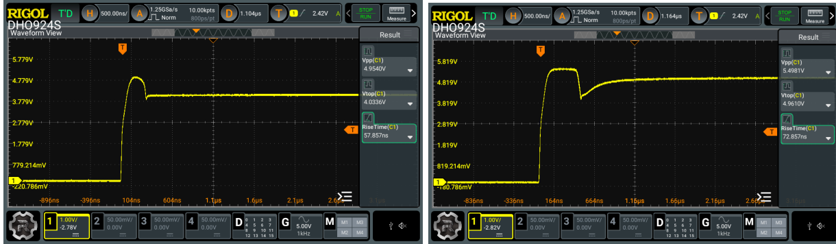
Zoomed in TP2 signal, LED on (left), LED off (right)
